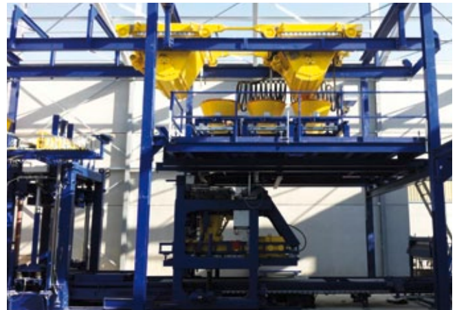
Assembly of the Premium colour mix system
