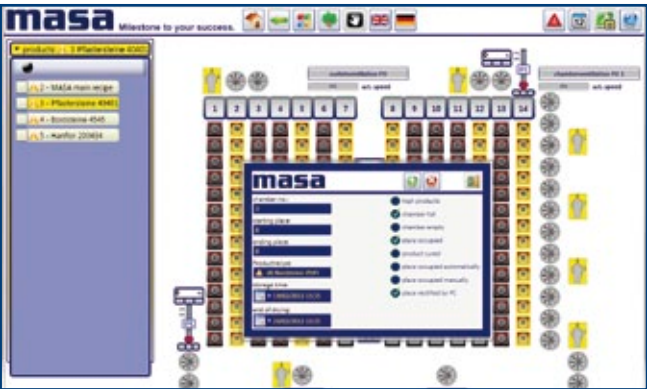
Masa FAST Factory Automation Service Tools: Curing Chamber assignment
