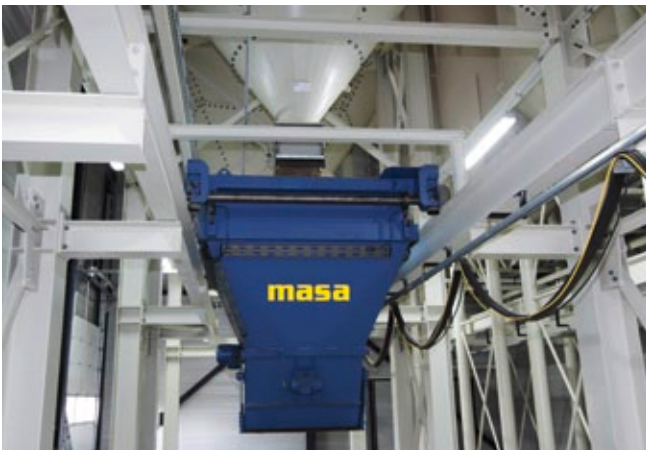
Exact dosing using moving charging scale
