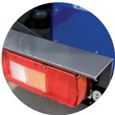
**Rear lights cover made of steel for avoiding damages.**
